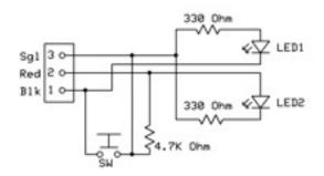
Fascia Controller Schematic for Single Color LEDS. 4.7K resistor is optional but will increase noise rejection. The switch is a NO (normally open) pushbutton type.
